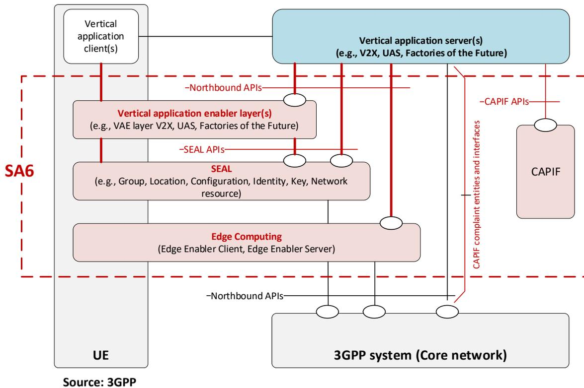
Figure 3-9: 3GPP vertical application enablement
