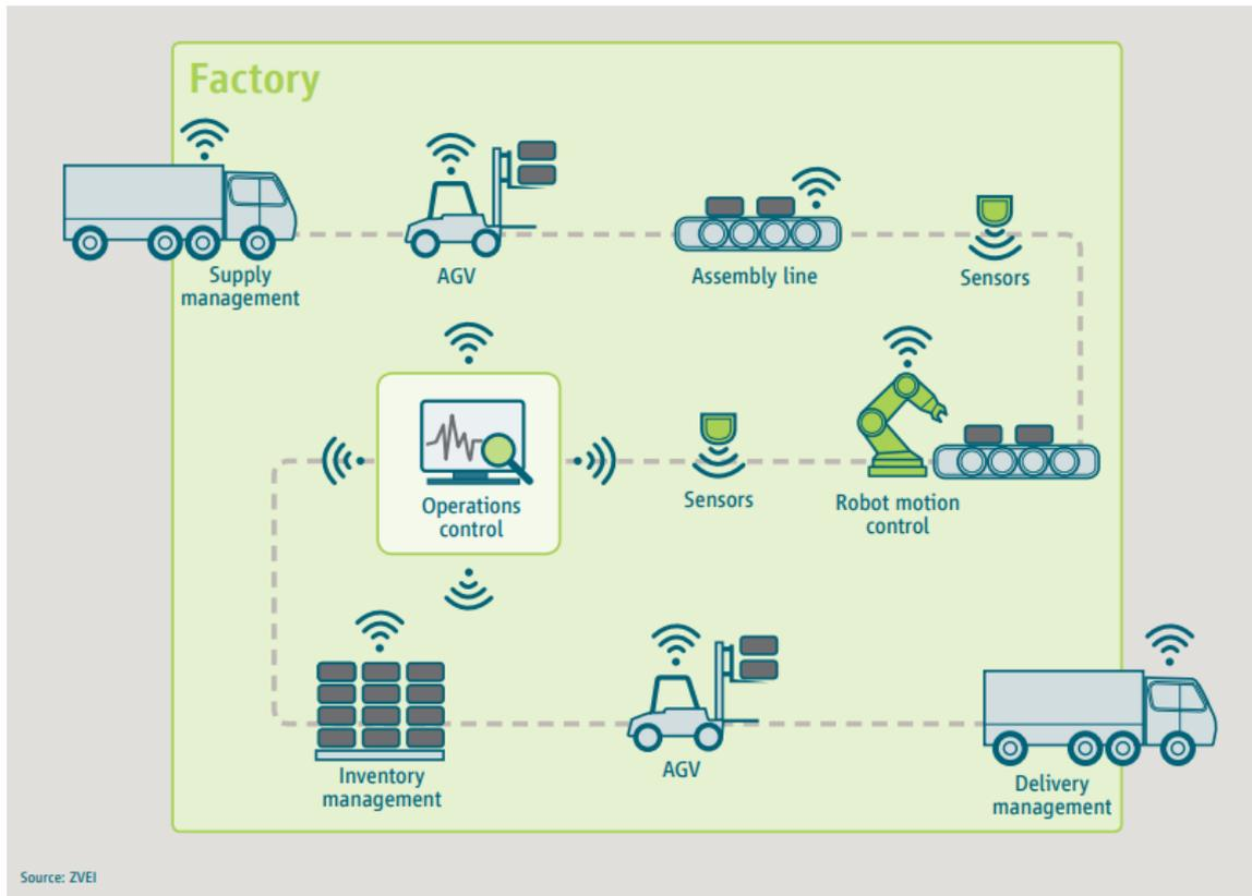
Figure 4-3: Applications of 5G in Smart Factory
